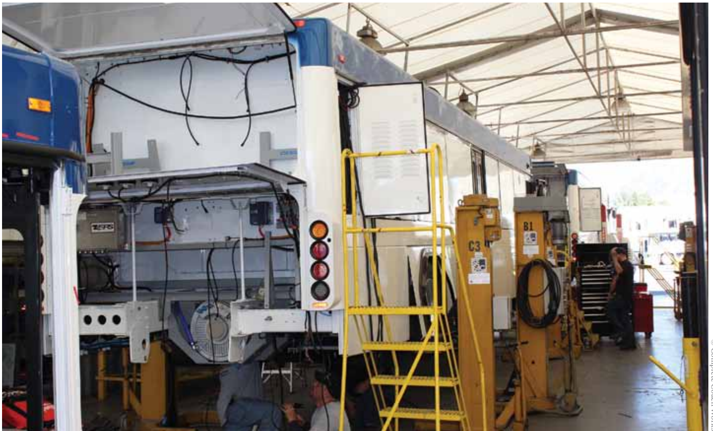
Complete Coach Works converts old diesel-run transit buses into buses that run on electricity, requiring both mechanical and electrical skills in its workforce.
