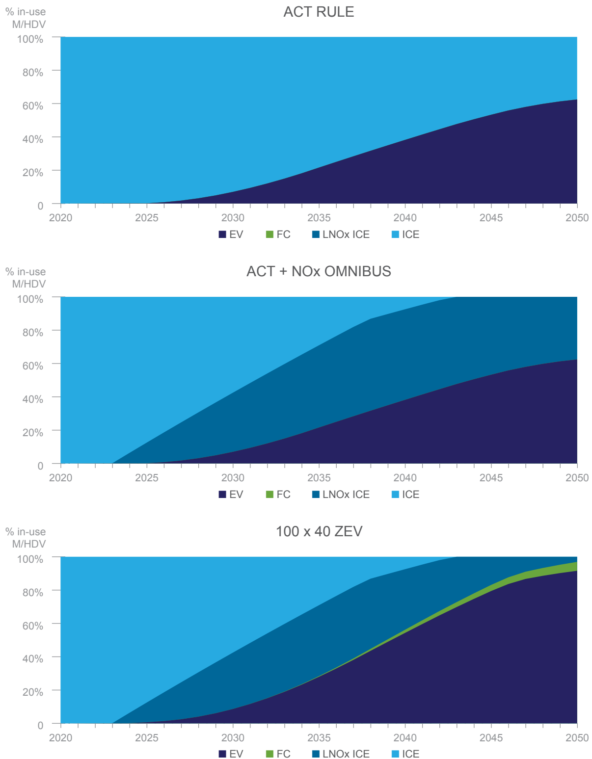
Figure 2 Fleet Turnover to Low-NOx and Zero-Emission Vehicles in Clean Truck Policy Scenarios
